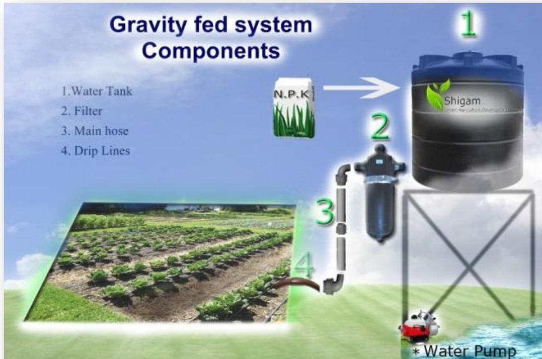
A gravity fed system is a good irrigation solution for small farms or plots which are not connected to the water system. It is mostly recommended for fields up to one acre. The idea is simple: Water mixed with soluble fertilizers in an elevated reservoir being gravitated down to the field where it will be distributed evenly using the drip tubes.
